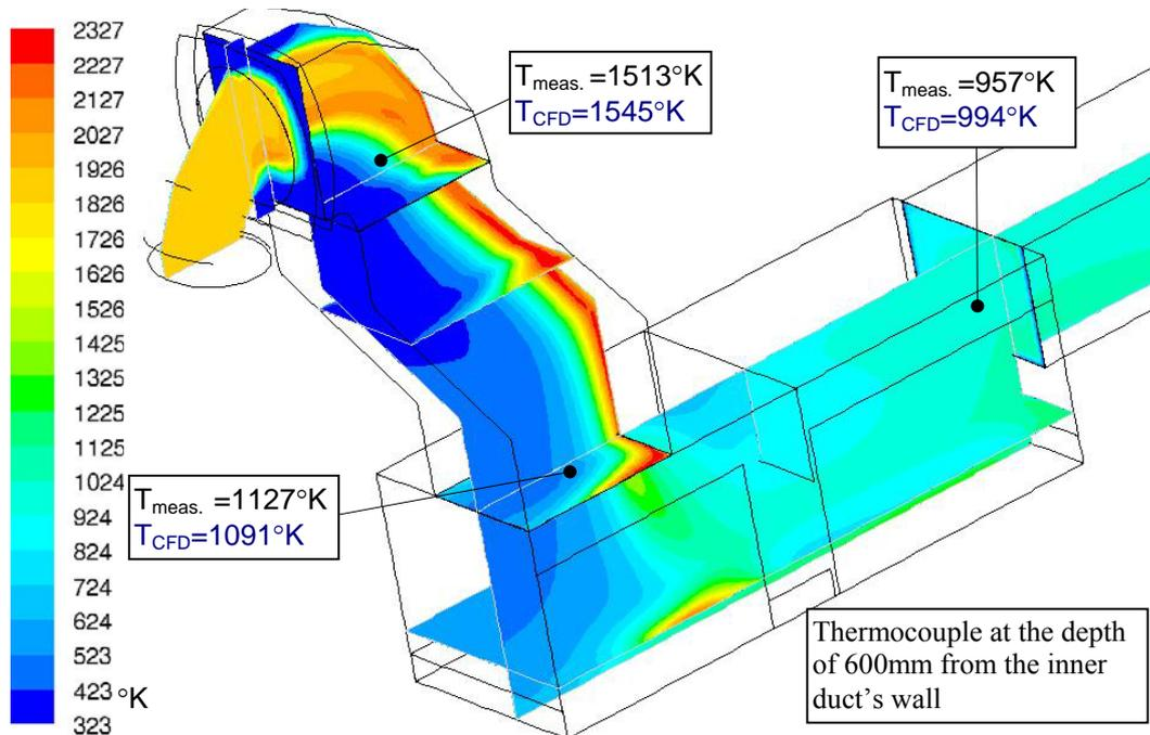
Figure 2. The temperature distribution range of the off-gases in the part from voltage joint to segment III (simulation I)
