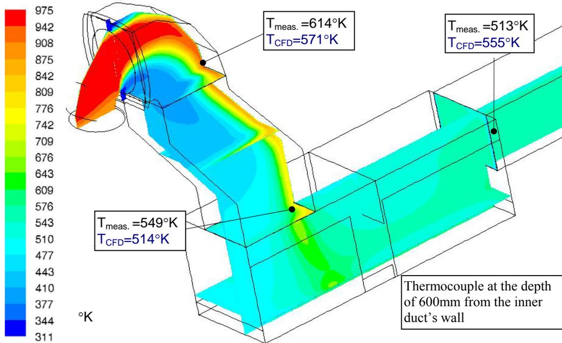
Figure 4. The temperature distribution range of the off-gases in the part from voltage joint to segment III (simulation II)
