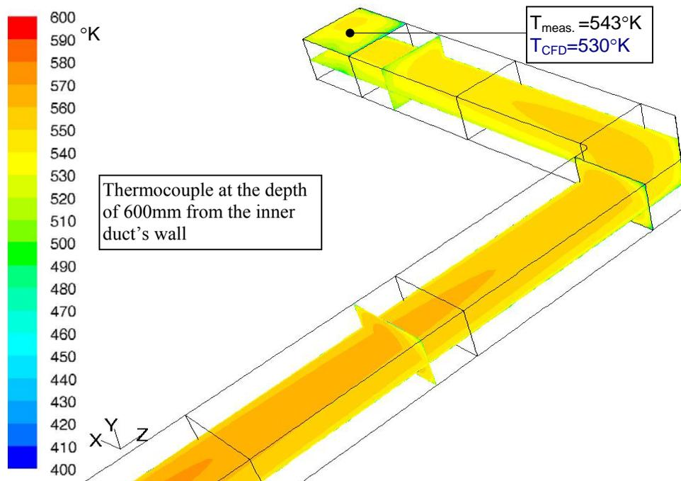
Figure 5. The temperature distribution range of the off-gases in the part from segment IV to the duct exit (simulation II)
