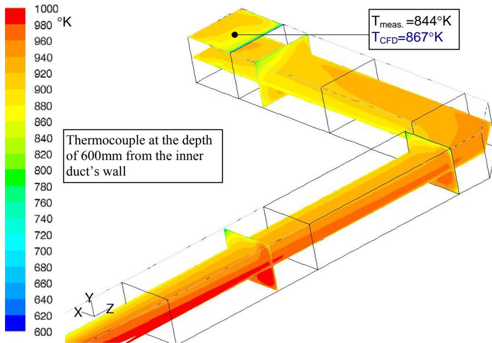
Figure 3. The temperature distribution range of the off-gases in the part from segment IV to the duct exit (simulation I)
