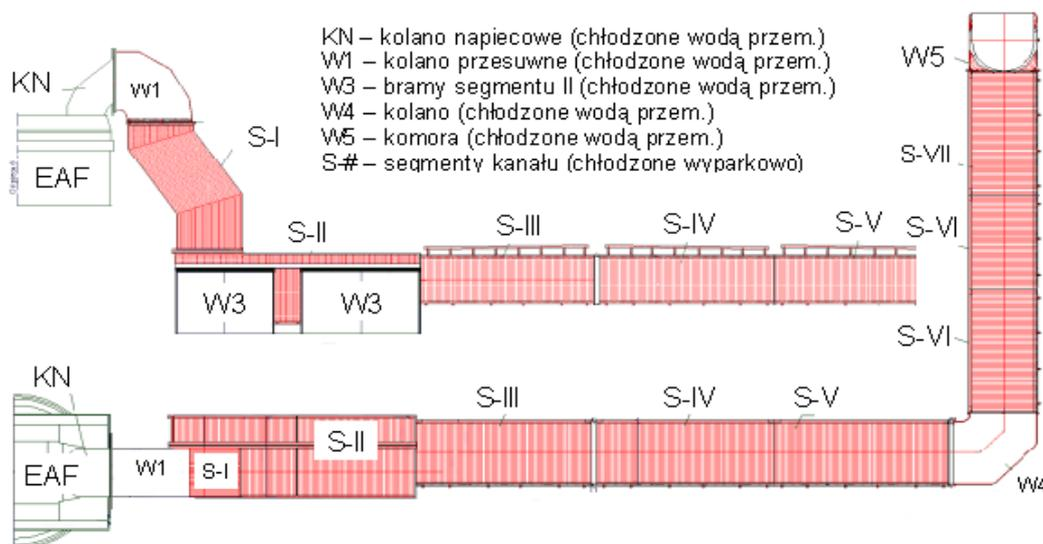
Figure 1. A simplified design of the off-gas duct of the arc furnace having the capacity of 140Mg.
